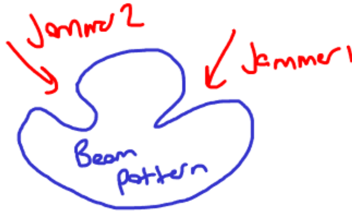
FIGURE 65.2. Jammer Signal Suppression with Sidelobe Canceller
